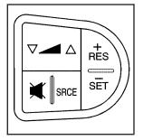
If your vehicle has this feature, some audio controls can be adjusted at the steering wheel.
